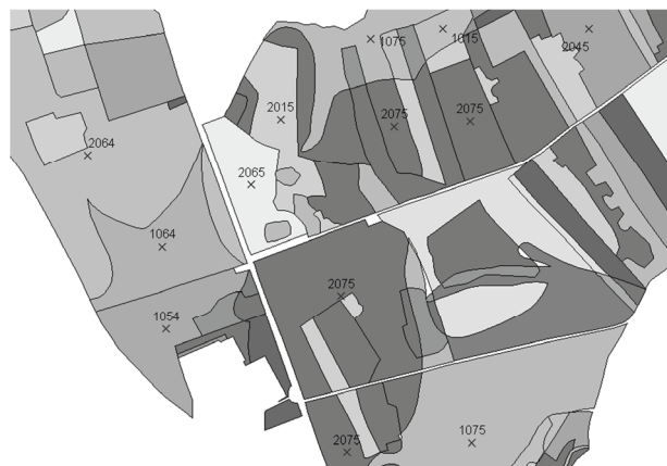
Fig. 3. Detail of the area stratification with generated sampling plots using randomized sampling (plot No. 2015 means that the plot is in site category 2, forest stand age 1–20 years, stocking above 9)
